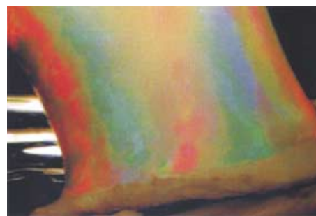
Figure 2. Photograph of a crosslinked polyacrylamide hydrogel in which polybutylacrylate colloids are immobilized. The occurrence of Bragg diffraction of the incident visible light indicates long-range order of the particles.
